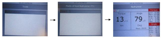
• Once the 5 tests are performed, confirm (or cancel) manually the new calibration coefficient on the CVI II (the new calibration coefficient is not sent automatically to the CVI II).
