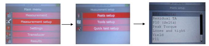
Press the *Valid* button on the Delta keyboard to *Modify/Delete* the selected *Pset*, or to create a new one:
