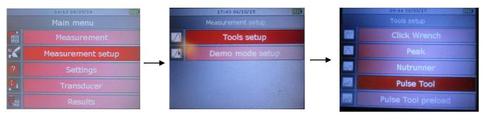
Delta 1D – Quick Test Setup
