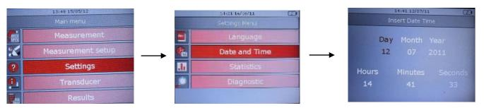
Use the *Left* and *Right* arrows on the keyboard to move in the menu, and the *Up* and *Down* arrows to increase and decrease the selected field.
