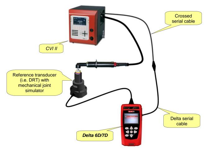
To connect the *Delta* and the *CVI II*, use the same cable to connect the Delta to the barcode reader, and a crossed serial cable to be connected to the serial port of the *CVI II*.
