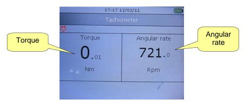
The tool can operate clockwise (angular speed is positive) or counterclockwise (angular speed negative).
