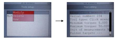
Scroll the parameters using the *Up/Down* keys and click on *Enter* to edit the parameter selected. Then set the value by means of the arrow buttons (left/right to select the digit, up/down to increase/decrease the value). Finally, either click on *Valid* to save or click on *Esc* to quit without saving.
