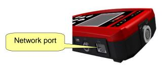
The Ethernet port can be used (as the USB port) for programming the Delta with the DeltaQC software. It is also possible to export test results on the Ethernet port.
