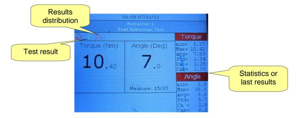
The test result is marked as OK (with icon) if the Cm and Cmk are greater than the minimum Cm and Cmk specified in the Pset; if not, it is marked as *Not OK* (with  $\bowtie$  icon).
