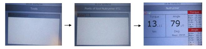
• Once the tests are performed, the CVI Monitor updates automatically the new calibration coefficient in the CVI3.
