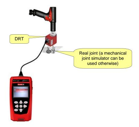
A DRT on the real joint (or a mechanical joint simulator) can be used. This also provides the angle measurement:
