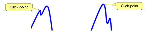
If the torque only drops down to zero (without increasing again) after a peak-point (as shown in the figure below), the click-point is not detected. For this reason, slip-wrenches cannot be tested with this method (slip-wrenches should be tested with the *Peak Test* (refer to the paragraph "*Peak Test*" for further details)):
