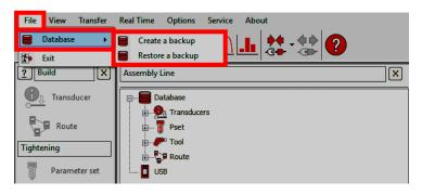
To create a database backup file, click on the tab  $File \rightarrow Database \rightarrow Create a backup$ . From the dialog box that opens (see the figure below):
