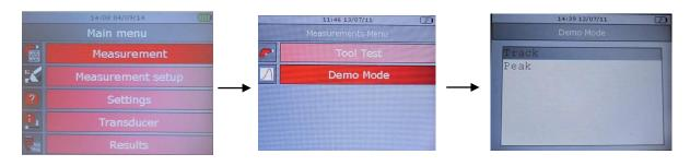
Delta 6D/7D: Select *Measurement* from the main menu; then select *Quick test*; finally select *Demo Mode*:
