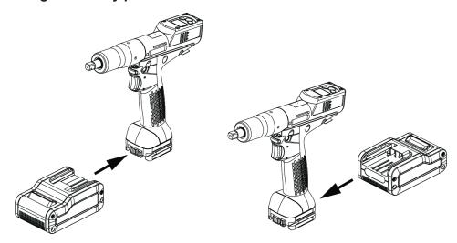
Insert the battery pack in front or behind the tool until a locking sound can be clearly heard.
