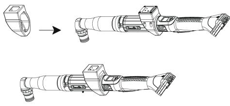
Slide the cover on the tool. Push it strongly over the reader.
