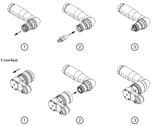
Plug an accessory into the quick-release output as shown and assign a Pset to it.
