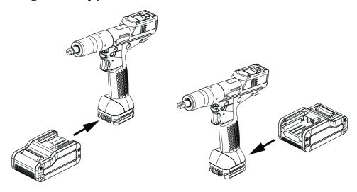
Insert the battery pack in front or behind the tool until a locking sound can be clearly heard.
