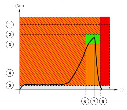
1 Abort torque 2 Max. torque 3 Min. torque 4 Angle threshold 5 Pset start torque Min. angle 6 Target angle
