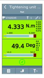
See in the screen above, the green anchor attesting that the system is working correctly.
