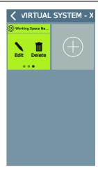
The working space for this tightening unit is done. Swipe the tile to the left to control that the tightening unit is correct. Swipe again to **Edit** or **Delete** the working space.
