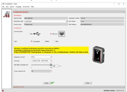
5. Select **USB** if the tracking base has to be connected physically to the USB port of CONNECT. Click **Write**.
