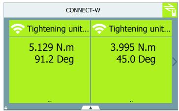
The green icon on the top right indicates the communication is established with the system.
