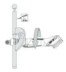
Use fixing clamps to tighten the angle head in the anticlockwise direction. Apply a torque of 50 Nm.
