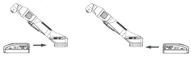
Insert the battery pack in front or behind the tool until a locking sound can be clearly heard.
