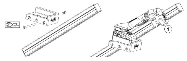
(i) Note above that an additional accessory (1) is required to hold the tool. This Desoutter accessory can be ordered as 6158114110.
