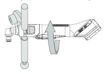
Use fixing clamps to unscrew the angle head in the clockwise direction.
