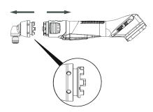
Disconnect the parts and locate the new position of the angle head.
