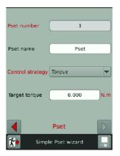
Tap the box **Target torque**.
