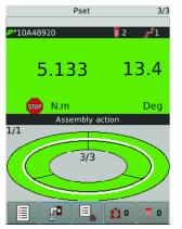
The process is finished and the report is OK. Assembly Process is set to 0 again. Pset is set to 0 again. The tool is locked, waiting for the next Assembly Process.
