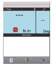
The **Stop** icon means that the tool is locked. The controller is waiting for the selection of a Pset to run the tool.
