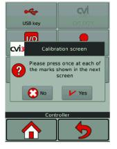
Tap **Yes** to display the calibration screen. Tap each of the 5 crosses. The controller will automatically re-calibrate the screen.
